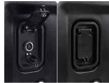
Deck power outlet
